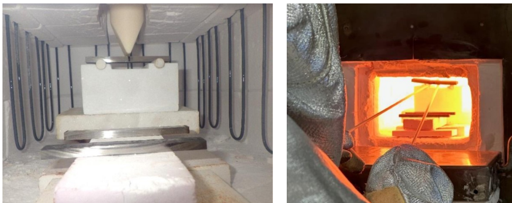
Figure 4. Hot modulus of rupture device. Left: at ambient temperature, Right: at 1 200 °C.
